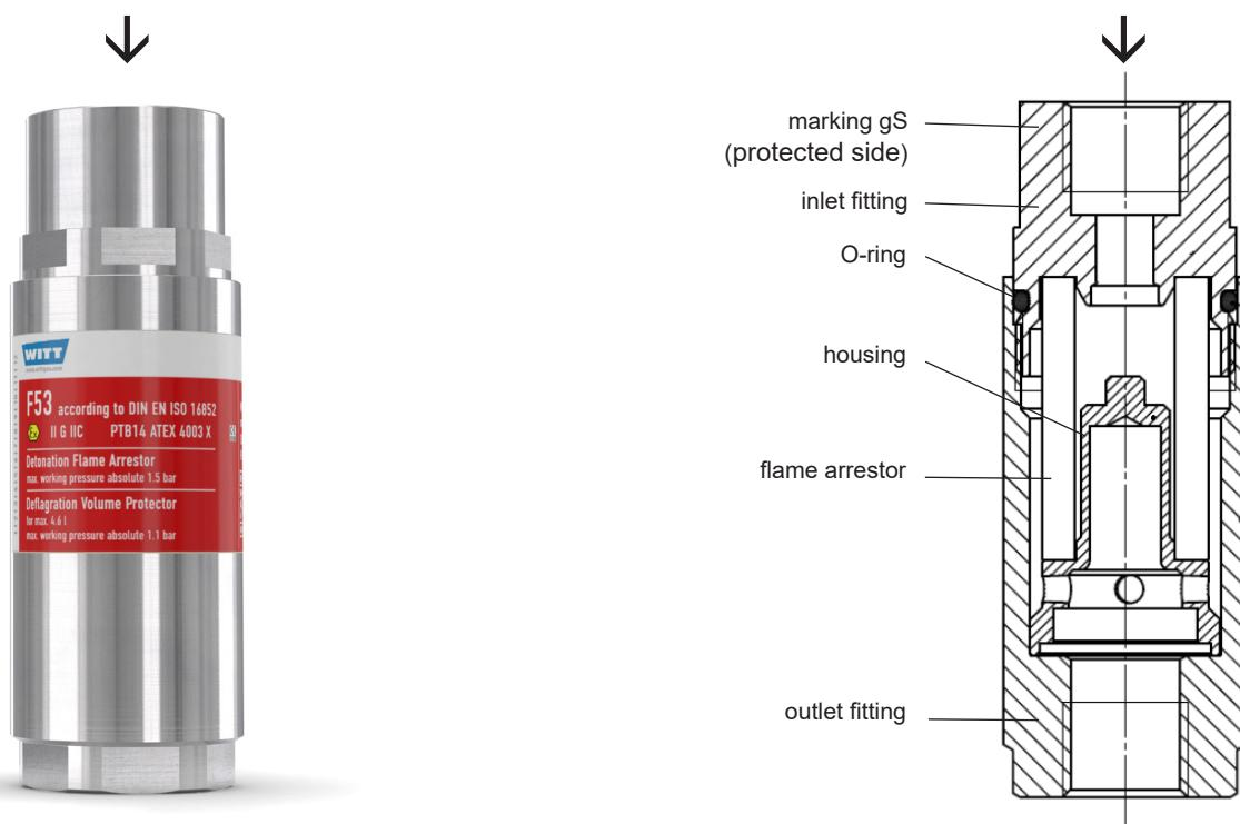
The deflagration volume protection device is ideal for protection of plants and equipment with a volume of max. 4.6 l.
