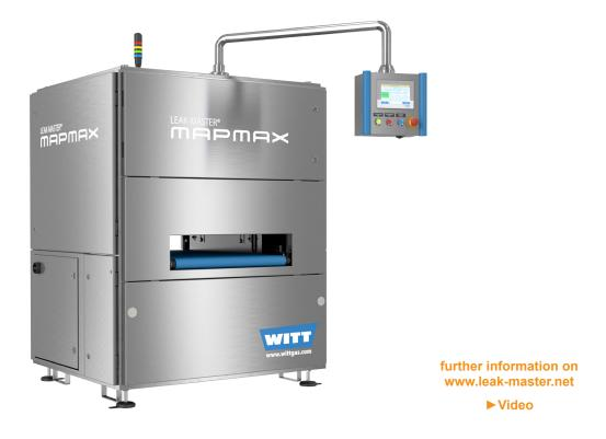
Automatic in-line micro-leak detection system for packages based on CO<sub>2</sub>. LEAK-MASTER® MAPMAX Compact features non-destructive detection of the smallest leaks without the need of costly helium - directly from the packaging line.
